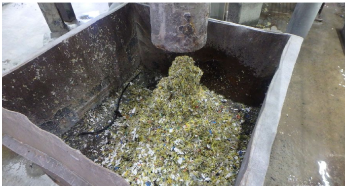
Mill trash screen separator overflow where we check for beads.
